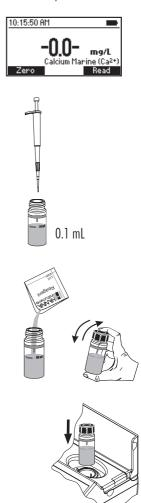
• Press Read to start the reading. The instrument displays the results in mg/L of calcium (Ca<sup>2+</sup>).
