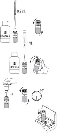
Press Timer and the display will show the countdown prior to zeroing the blank or wait 2 minutes and then press Zero. The display will show "-0.0-" when the meter is zeroed and ready for measurement.
