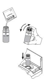
• Press **Timer** and the display will show the countdown prior to the measurement or wait 1 minute and press **Read**. When the timer ends the meter will perform the reading. The instrument displays the results in **mg/L** of **chlorine (Cl<sub>2</sub>)**.
