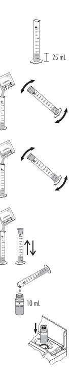
Press Timer and the display will show the countdown prior to the measurement or wait 5 minutes and press Read. When the timer ends the meter will perform the reading. The instrument displays concentration in mg/L of molybdenum (Mo<sup>6+</sup>).
