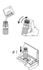
• Press **Timer** and the display will show the countdown prior to the measurement or wait 2 minutes and 30 seconds and press **Read**. When the timer ends the meter will perform the reading. The instrument displays the concentration in **mg/L** of **Iodine (I**<sub>2</sub>).
