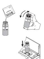
• Press **Timer** and the display will show the countdown prior to the measurement or wait 2 minutes and press **Read**. When the timer ends the meter will perform the reading. The instrument displays the result in **mg/L ozone (O**<sub>3</sub>) (chlorine free sample only). For samples containing chlorine, record this value as A.
