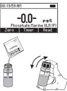
• Insert the cuvette into the holder and close the lid.
